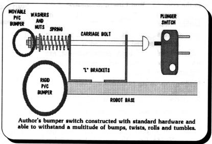
some time to ensure smooth sliding of the carriage bolt. The switch used in this example is a standard plunger-style made by Microswitch.
