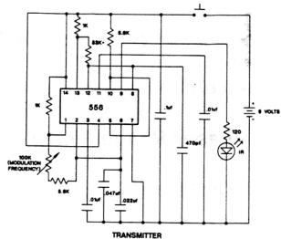
\*Ground Pin 6 and adjust for 40 kHz ± 2 kHz from Pin 9 with
