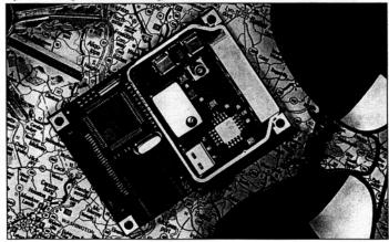
shock and vibration conditions. Further, new power management circuitry reduces the receiver's average power dissipation to 670 mW. And a differential GPS option can improve accuracy from 100 meters to 5 meters 95% of the time. MicroTracker costs \$480 each/200 and operates with inexpensive passive antenna. ROCKWELL INTERNATIONAL CORP., P.O. Box C, Newport Beach, CA 92658-8902. (800) 436-9988
