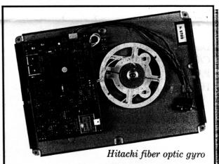
The Hitachi Optical Fiber Gyro is for automotive navigational systems. It detects vehicle rotations, and a one-chip microcomputer analyzes the data to provide the vehicle's azimuth.
