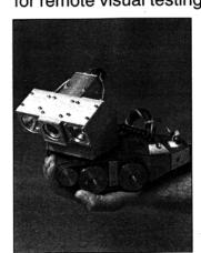
Miniature, waterproof, pan-and-tilt S-VHS Rovver is designed with remote control iris, two 35 W lamps, and onboard color CCD camera with over 375,000 pixels and S-VHS and composite video output. Imaging technology ensures good picture clarity in live and playback modes. Lazrlyne measurement capabilities allow for calculation
