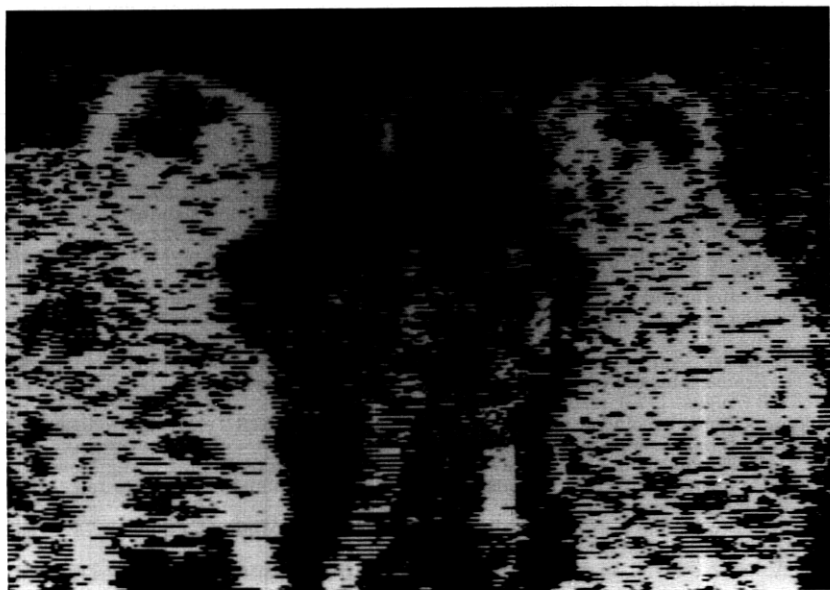
Fig. 7—Regions of different predictor use by the gain- and displacement-compensated coder for the frame of Fig. 5. Bright pels correspond to displacement-compensated predictor [ P_3 of eq. (26)], light pels correspond to gain-compensated predictor [ P_2 of eq. (26)], and dark pels correspond to previous frame predictor [ P_1 of eq. (26)]. It is seen that unchanging background areas use the previous frame predictor, and most of the shadow regions use the gain-compensated predictor.
