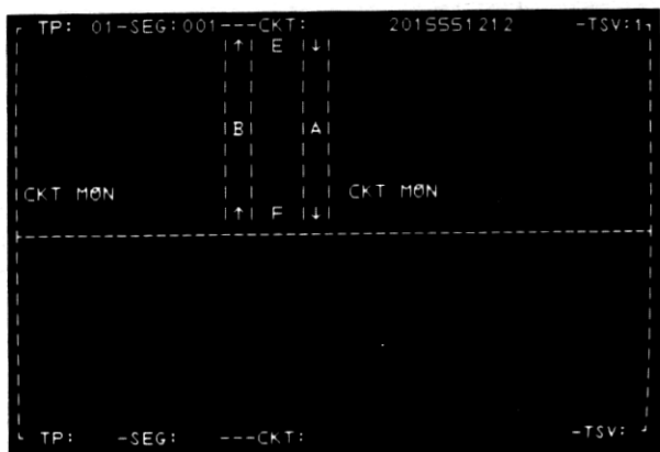
Fig. 7—4-wire circuit test point area display.
