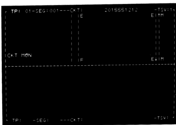
Fig. 8—2-wire E&M circuit test point area display.
