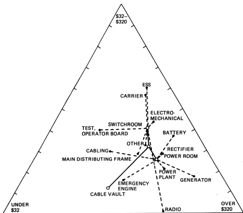
Fig. 6—A trinomial distribution of telephone equipment fire damage.
