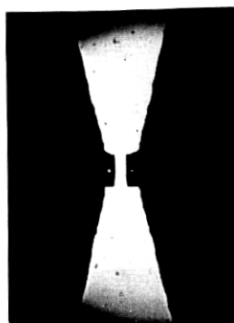
Fig. 10—Shadowgraph of opposing fiber ends of two plugs mated in the socket of Fig. 9.
