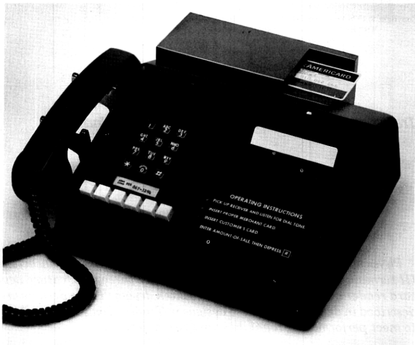
Fig. 1—Transaction telephone used in field trial.
