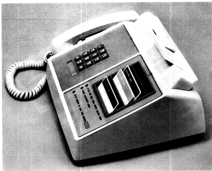
Fig. 6—Transaction set with first slot reader.
