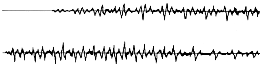
(b) CVSD-CODED WAVEFORM ( G = 1.264 )
