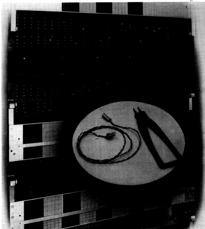
Fig. 7—Cross-connect panel, jumper, and removal tool.
