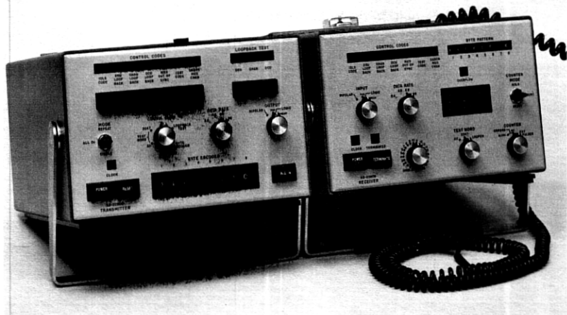
Fig. 6—Digital transmitter and receiver test sets.
