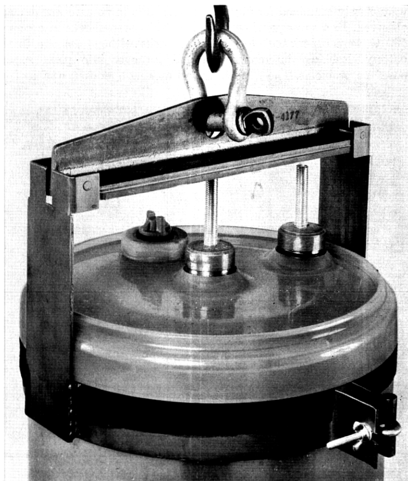
Fig. 10—Clamping fixture for lifting cell by its cover.
