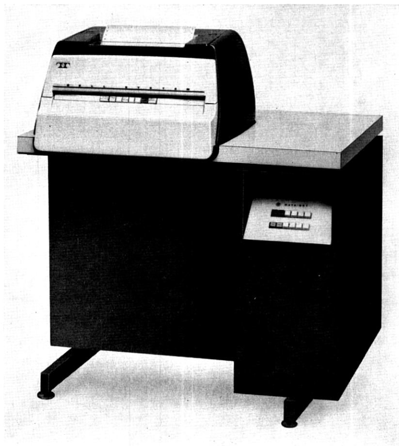
Fig. 9—Model 37 RO teletypewriter.
