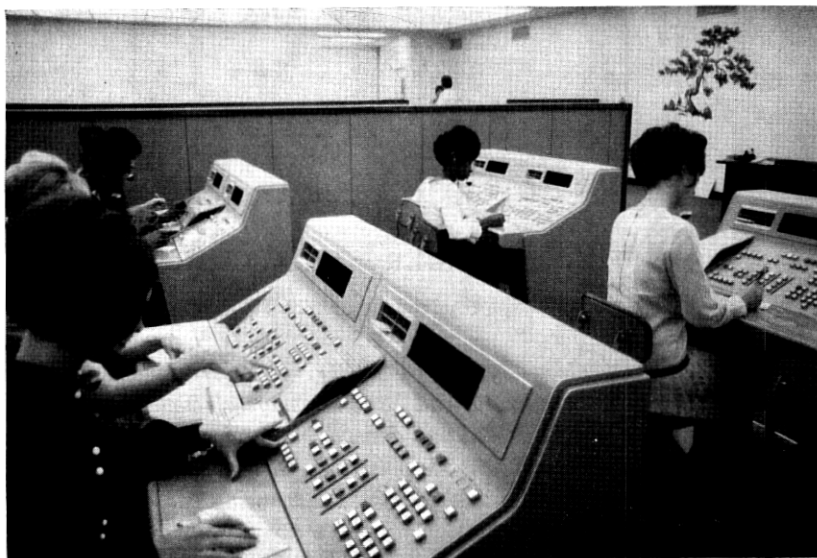
Fig. 1—Portion of a chief operator unit, TSPS No. 1.
