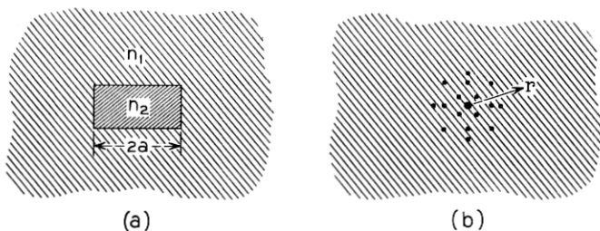
Fig. 1 — Waveguide cross sections: (a) rectangular shape, index n_2 > n_1 , (b) round shape.
