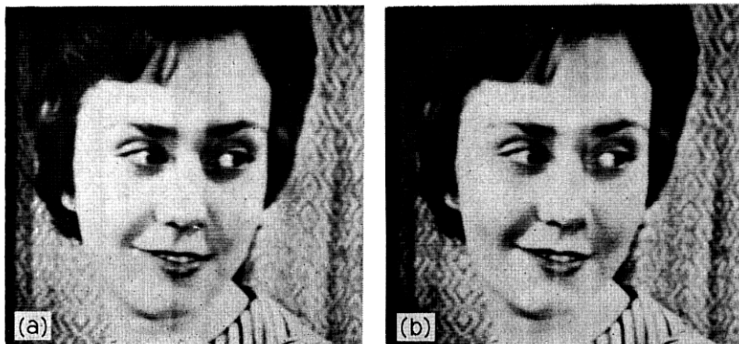
Fig. 11—Effect of transmitting erroneous \pm d' word when the erroneous word is locked to the scanning rates: (a) -d' error, (d) +d' error.
