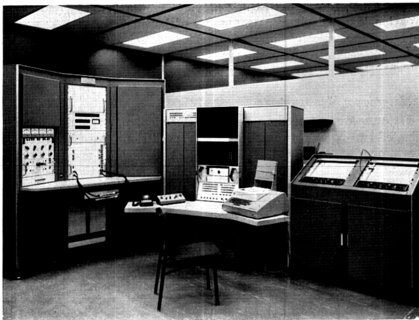
Fig. 1—Computer-operated transmission measuring set.
