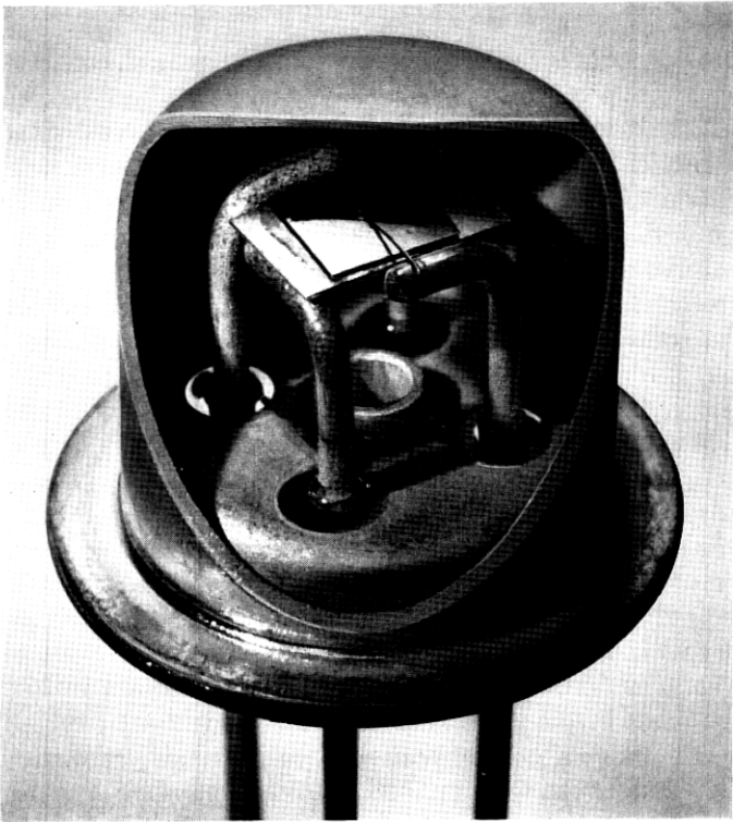
Fig. 6 — Construction of the radiation damage transistors.
