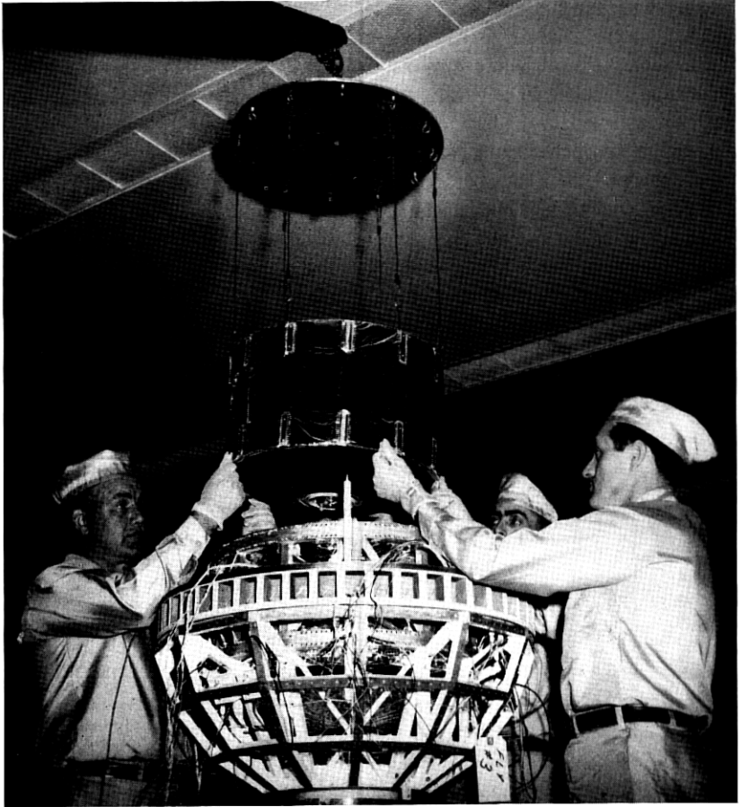
Fig. 9 — Mounting of electronics canister into the frame.
