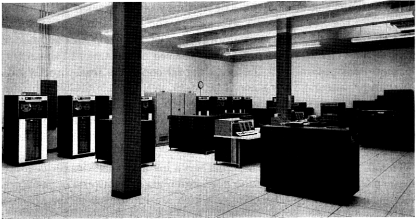
Fig. 2 — Two computing systems with four tape units each; three cabinets between tape units contain tape switching equipment.
