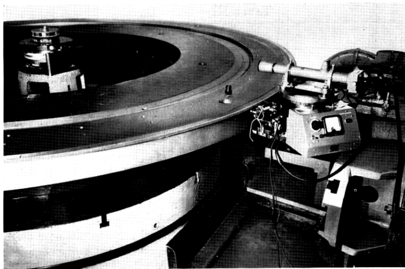
Fig. 11 — Test equipment for checking errors in gear tooth flank angular position.
