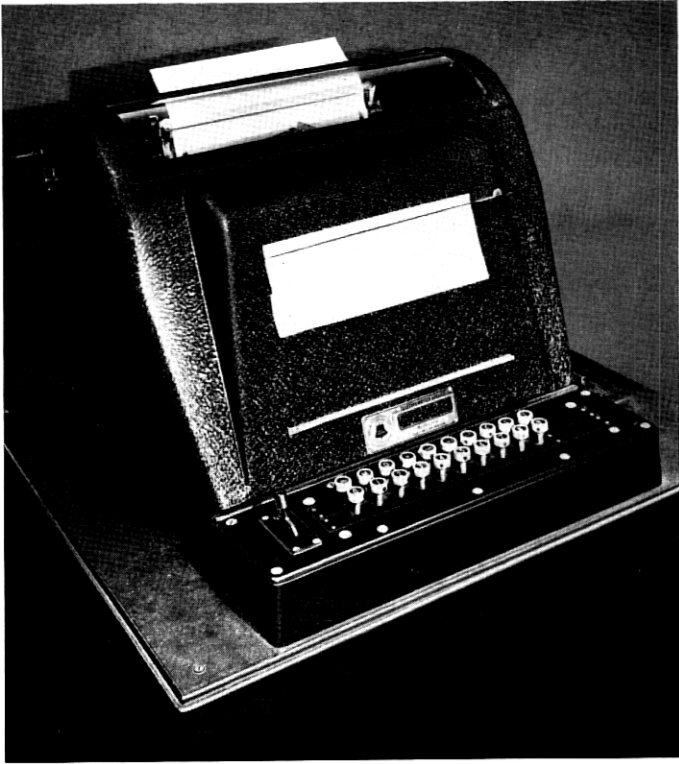
Fig. 1 — One of the three operator stations of the Complex Computer.
