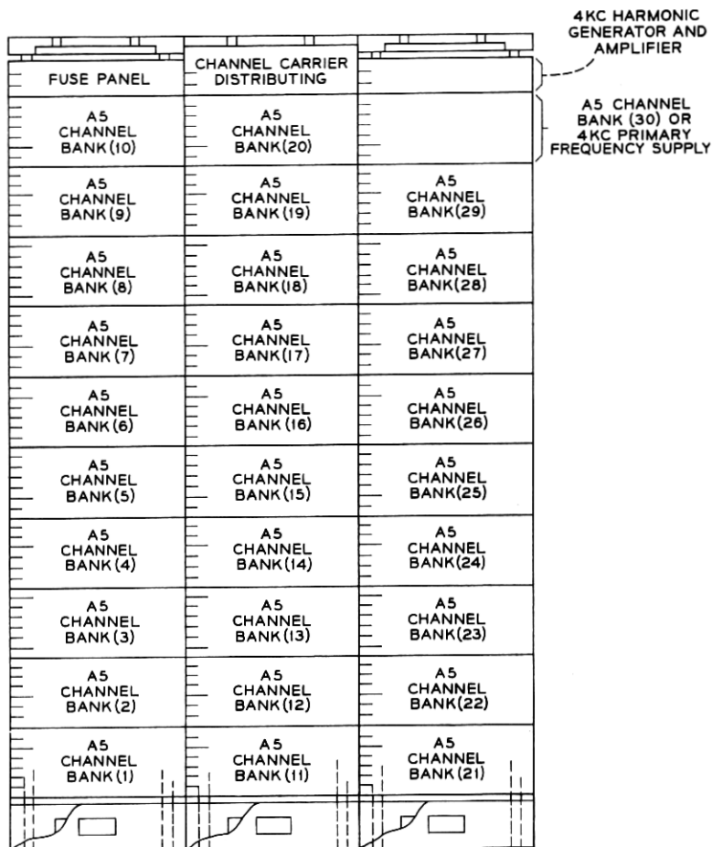
Fig. 18 — Arrangement for 30 A5 channel banks and associated carrier supply.
