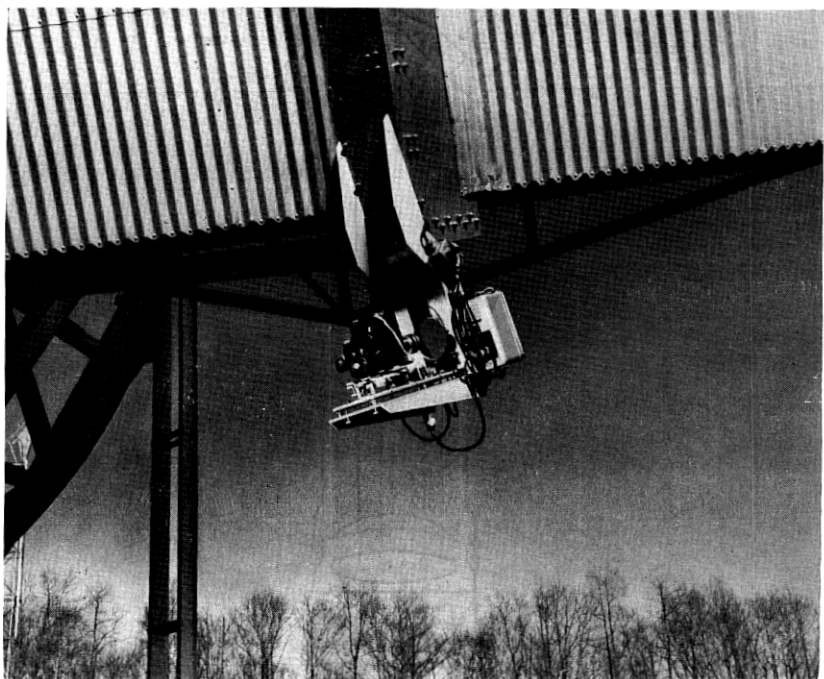
Fig. 4 — Camera mounted on horn receiver.
