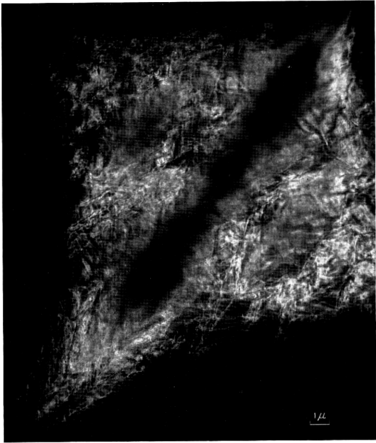
Fig. 5 — Electron interference effects in dark-field micrograph of crystal aggregate. Note the profusion of extinction lines and curves.
