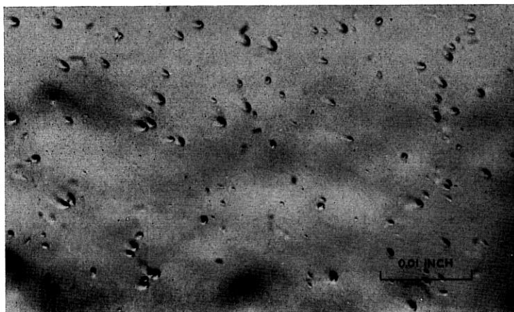
Fig. 3. — Microphotograph of Typical Etch Pits on (111) Plane.
