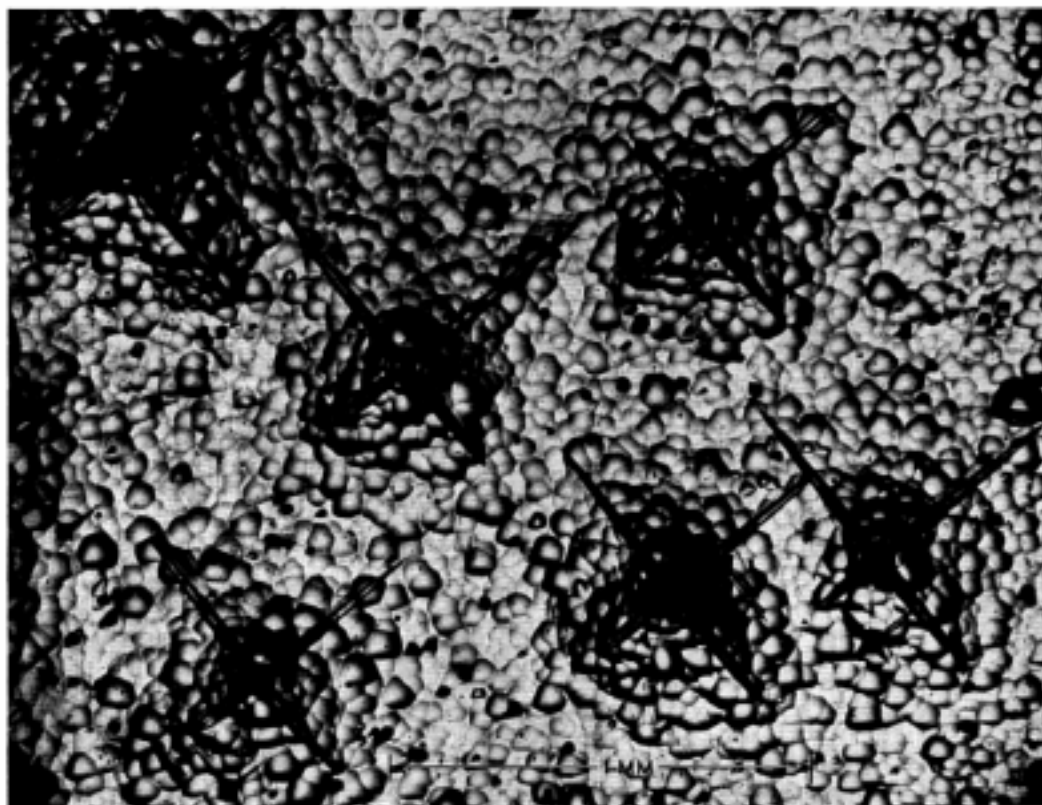
Fig. 7 — Electrolytic etch pits on n-type germanium.
