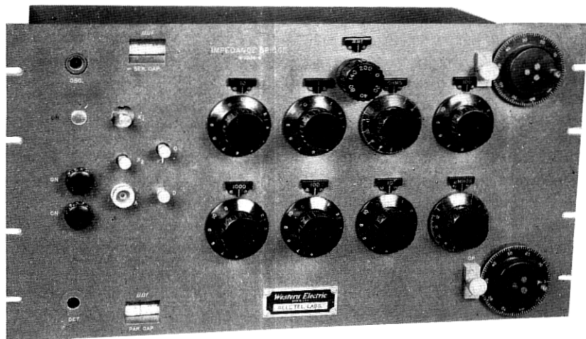
Fig. 6—Front view of the general-purpose bridge shown in Fig. 5. The bridge is approximately 10½ inches high and 19 inches wide.
