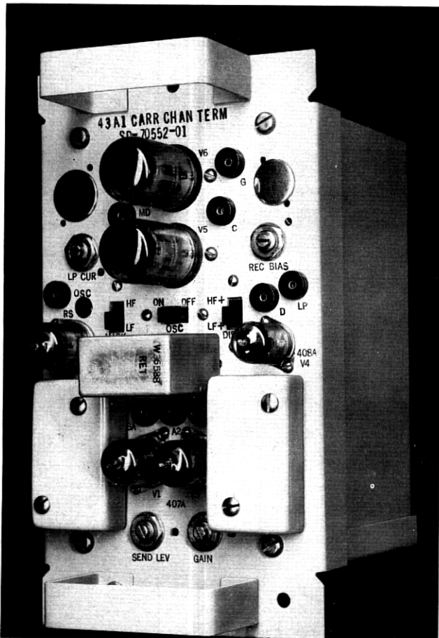
Fig. 7—Channel terminal, front view.
