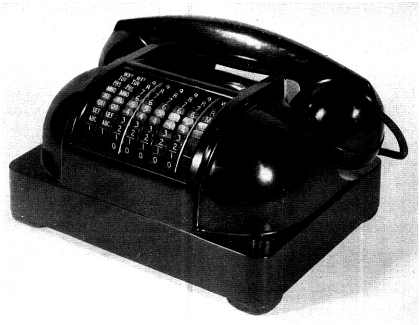
Fig. 5—Pre-set pulse-position-dialing telephone set.
