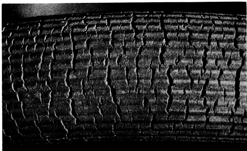
Fig. 5—Samples of rubber garden hose cracked by ozone.
