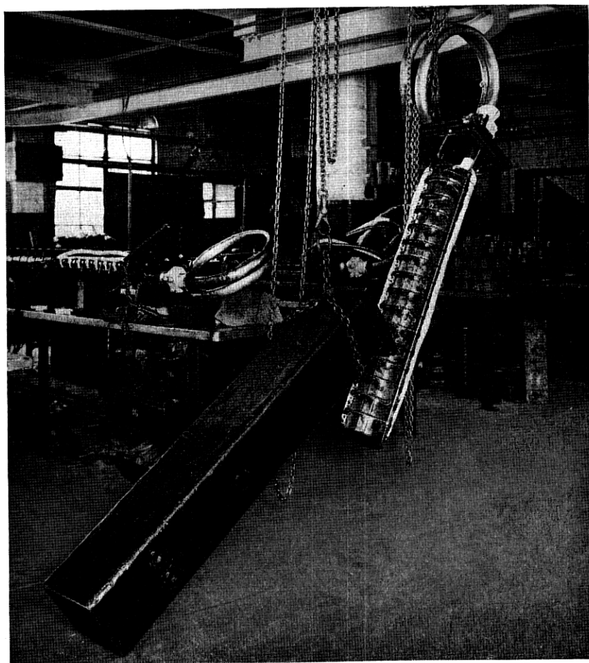
Fig. 30—Various stages in the assembly of toroidal type carrier loading coils. Several coils mounted in their shielding containers are piled on a bench at right center. On the bench at left center, an assembly of coils is being connected to the stub cable conductors. In diagonal center, a completely assembled and cabled complement of 16 coils is ready for placement in a tall, rectangular shaped, cast iron case.
