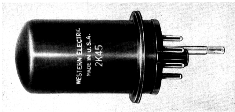
Fig. 75.—An external view of the W.E. 2K45—an early thermally tuned reflex oscillator designed by the Bell Telephone Laboratories.
