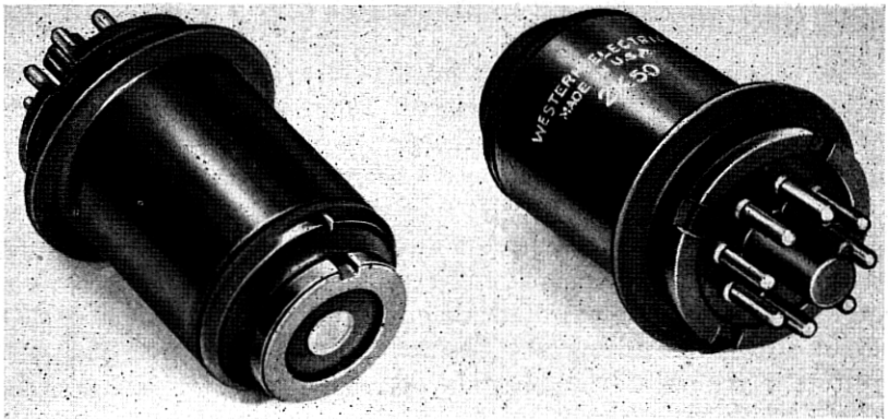
Fig. 89.—The 2K50—a reflex oscillator with thermal tuning and a wave guide output or operation in the 1 centimeter range.
