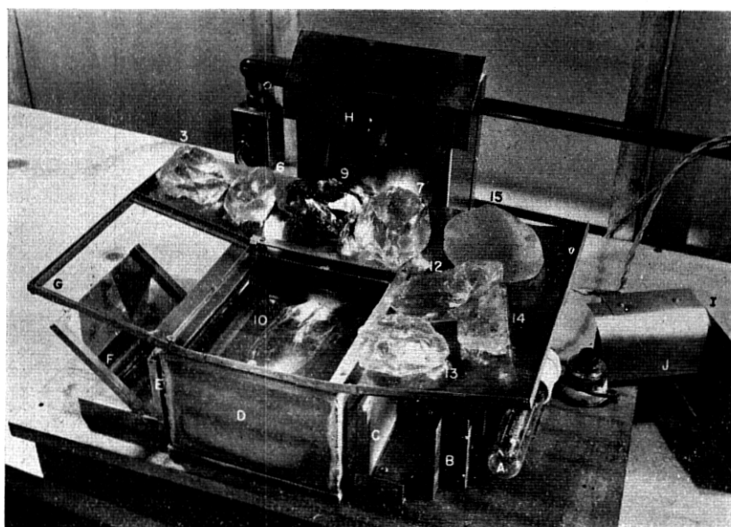
Fig. 4.5—The inspectoscope and stones used for the following figures. See also Fig. 4.3
