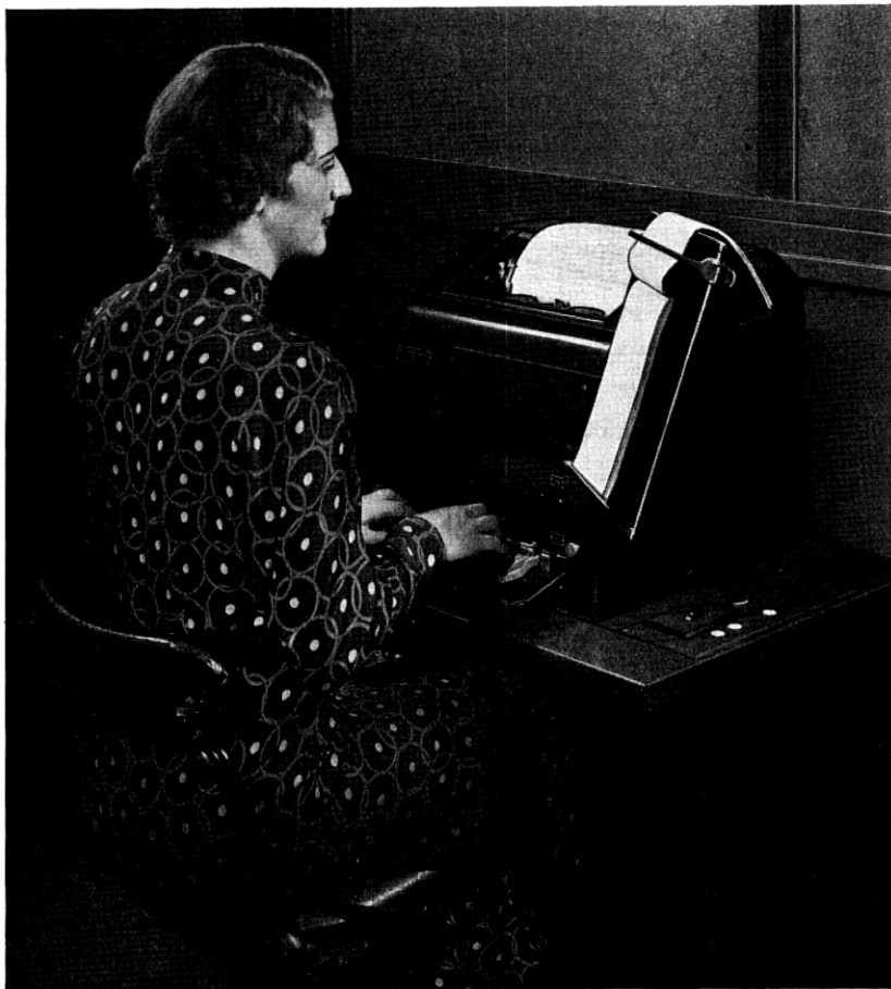
Fig. 9—Typical teletypewriter subscriber equipment for attended service.
