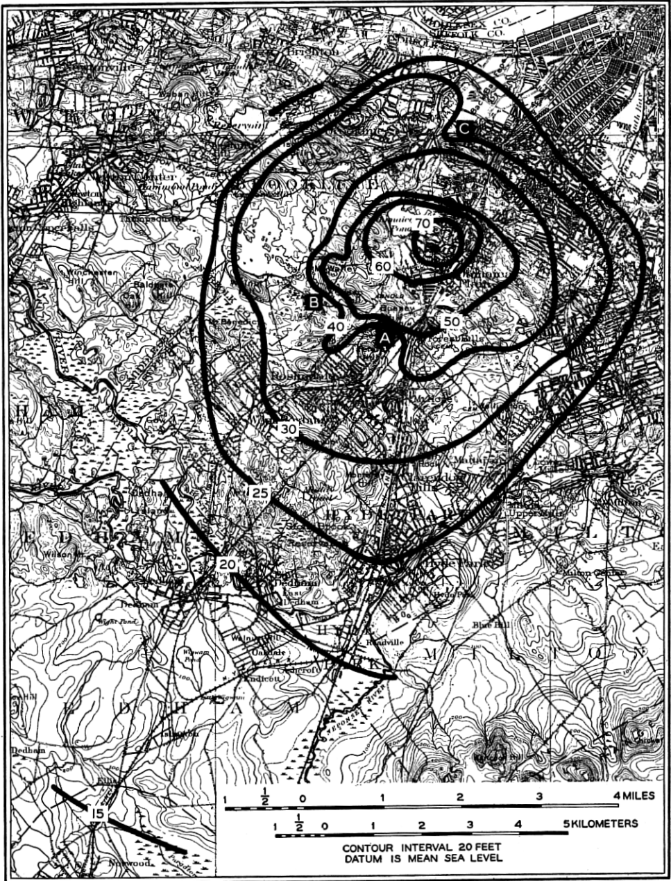
Fig. 11—Field strength contour map of Boston, Mass. Receiver located on Seaverns Street near Center Street as shown by the solid circle. Frequency = 34.6 mc. Field strength in decibels above one microvolt per meter.
