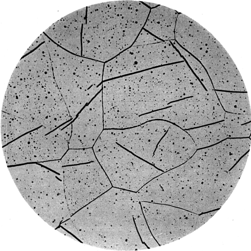
Fig. 20—The same alloy as shown in Fig. 19 after a subsequent aging treatment of 5 hours at 725° C. Mag. 125 X.
