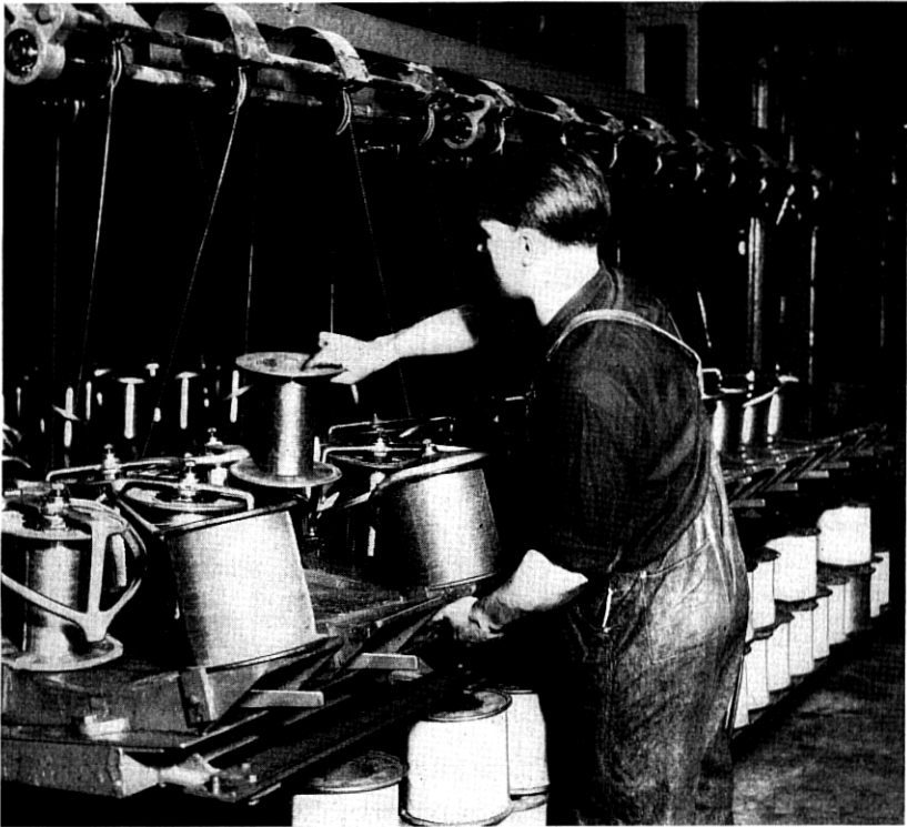
Fig. 4—Changing spools at supply end.
