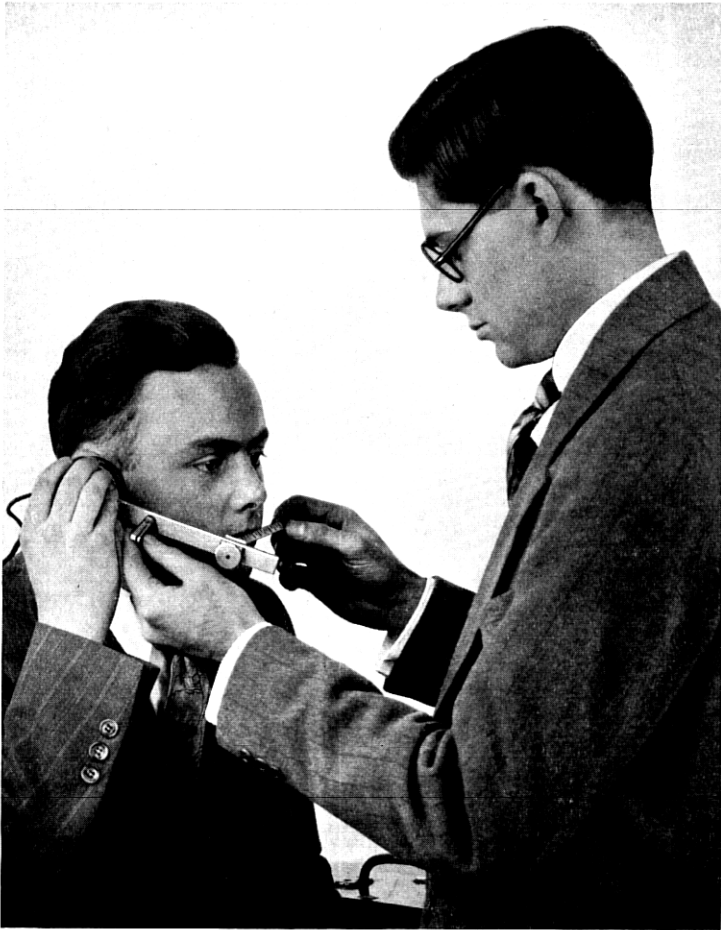
Fig. 10—Use of gauge for head measurements.
