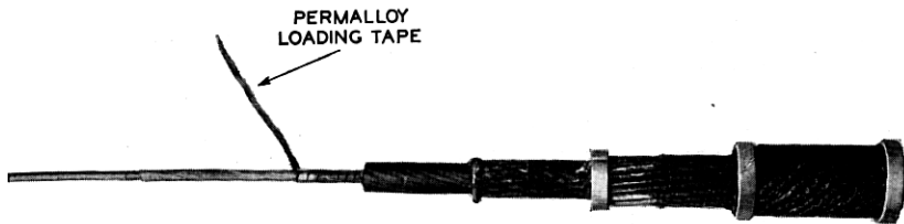
Fig. 21—Sample of submarine loaded cable, showing the loaded conductor.
