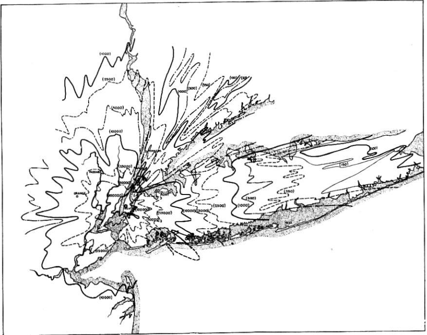
Fig. 4—Field strength contour map of distribution over the New York metropolitan area, effected by Station WEAJ. 5 kilowatts in antenna, frequency 610 kilocycles, wave-length 492 meters.
