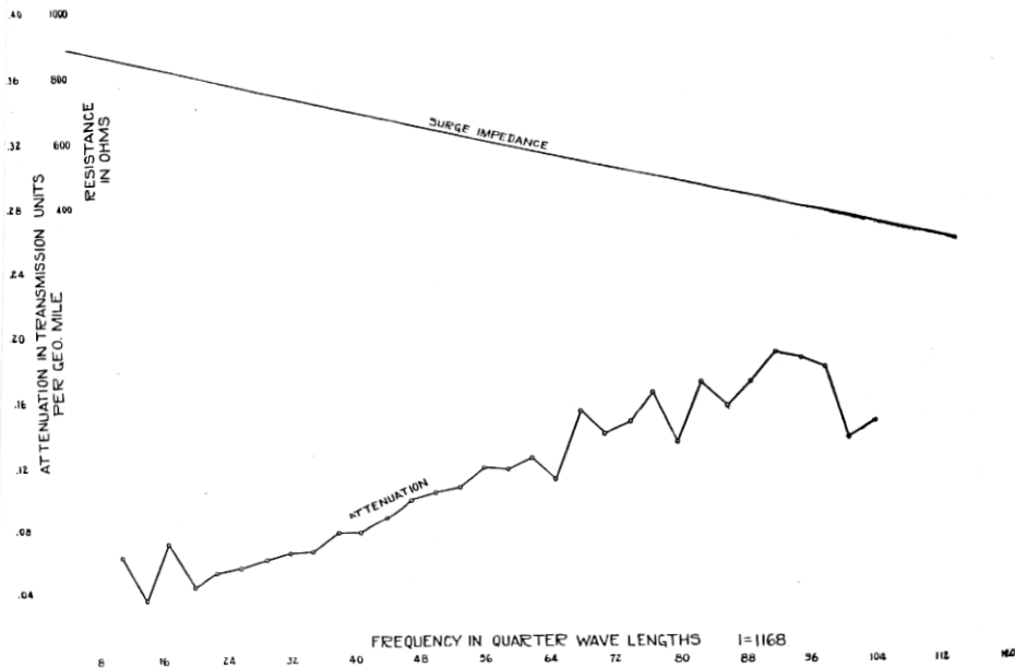
Fig. 3—Frequency vs. Attenuation and Frequency vs. Surge Impedance as Measured on the Tallulah Falls-Gainesville 110,000 Volt Power Line
