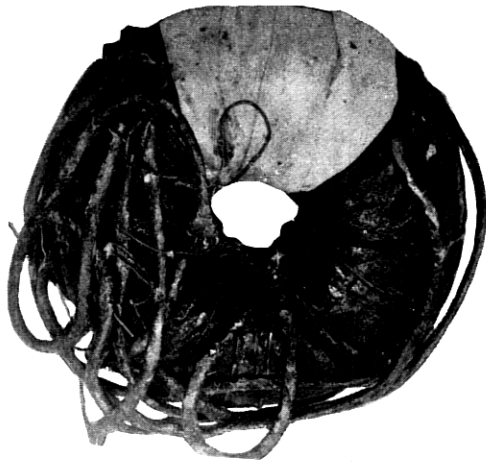
Fig. 18—Loading Coil with Winding Completed
