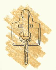
You can temporarily rest the handset in the cradle vertically on the front of the set if you have to leave the phone in the middle of a call.
