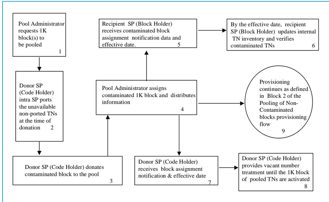
**Figure 3-2. Pooling of Contaminated Block**
