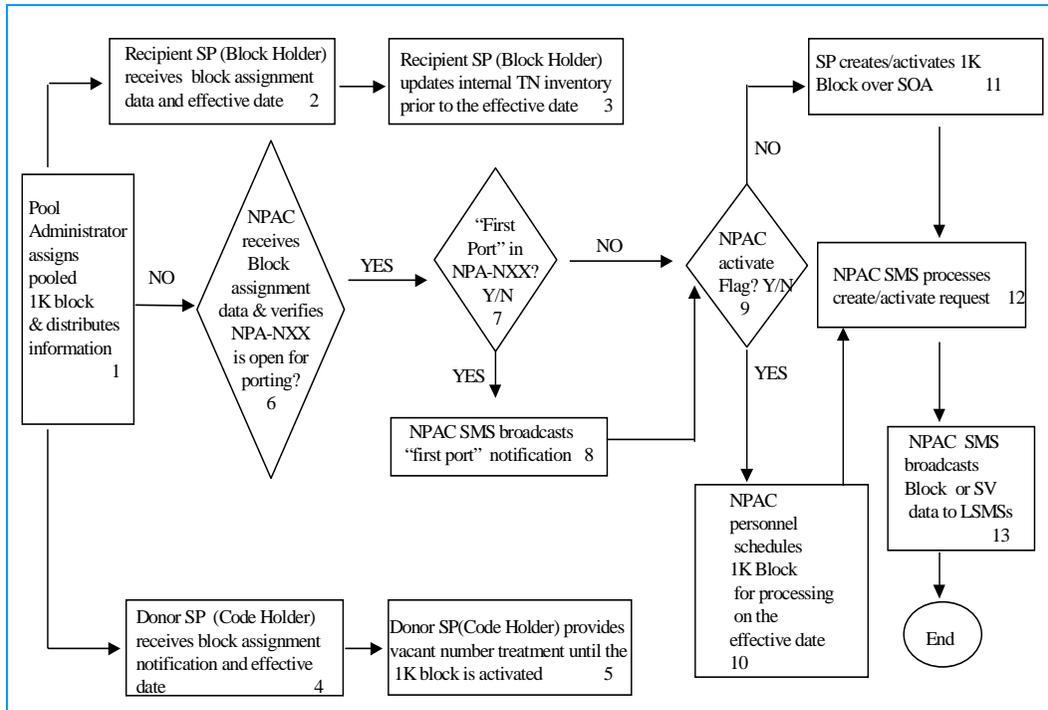
Figure 3-1. Pooling of Non-Contaminated Block
