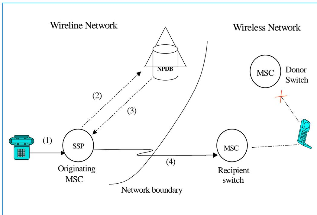
**Figure 2-13.** Call Completion from Wireline to Ported Wireless
