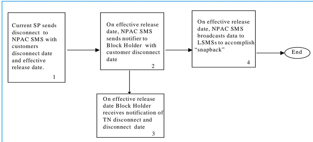
**Figure 3-4.** Disconnect of Ported Pooled Number
