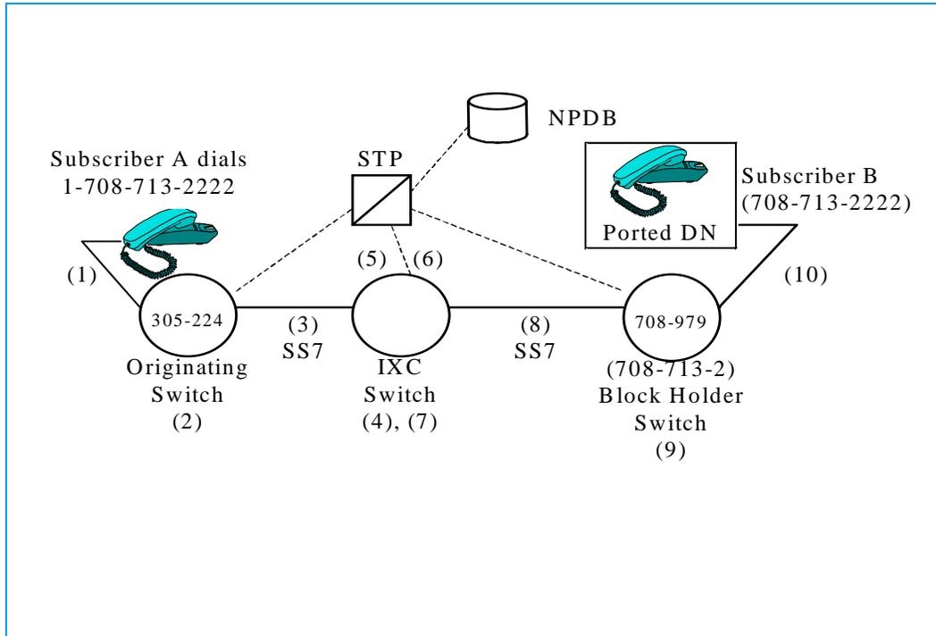
**Figure 3-8.** Call Completion Through an IXC
