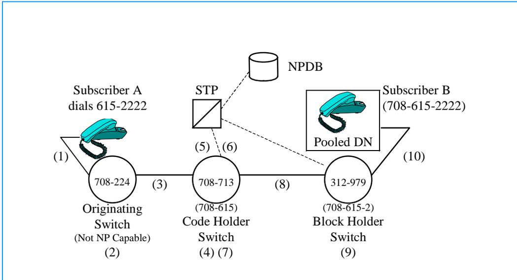
**Figure 3-7. Call Completion Via Code Holder Switch**
