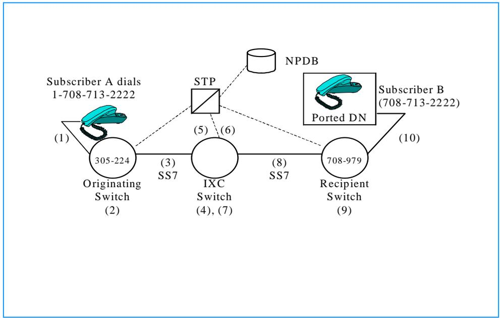
Figure 2-11. IXC-Routed Call; NP Query at IXC (N-1) Switch
