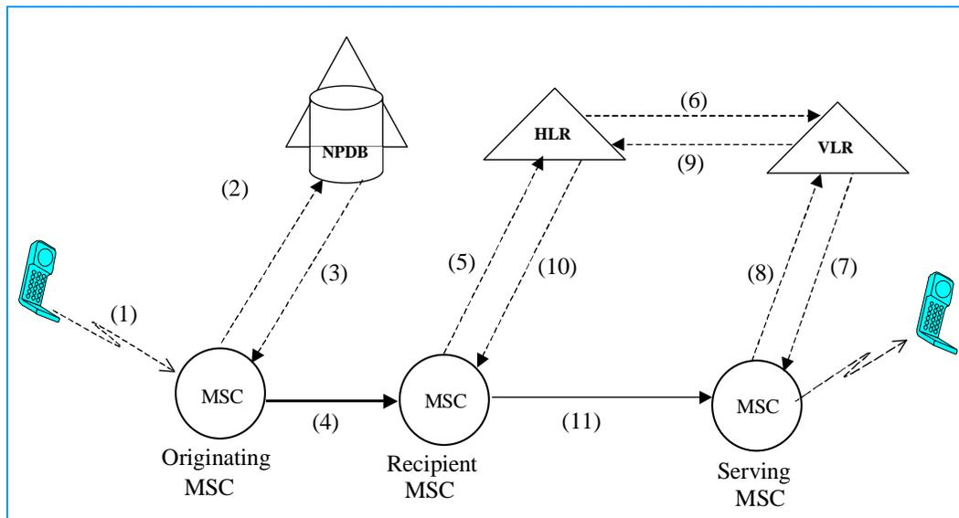
**Figure 2-15.** Call Completion to Roaming Ported Wireless User
