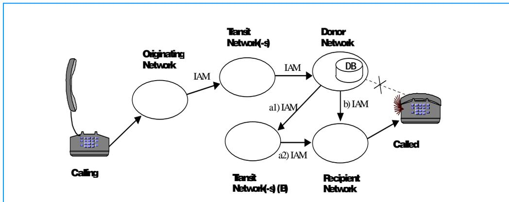
Figure 2-17. ITU Illustration of Onward Routing
