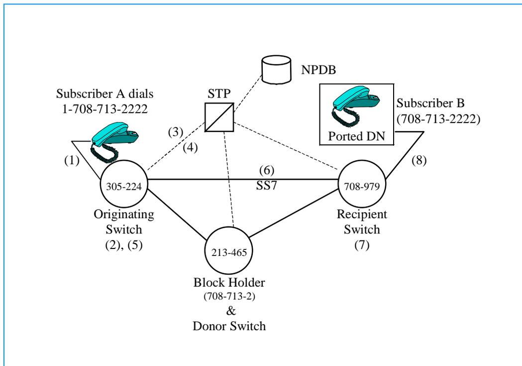
**Figure 3-9.** Ported Number in a Pooled Block
