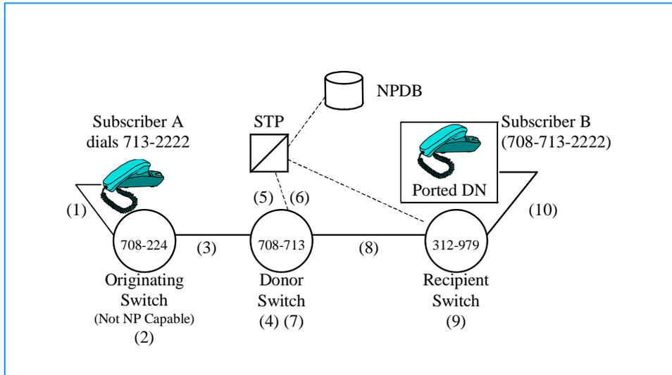
**Figure 2-10.** Call Completion via the Donor Switch, with a Donor Switch NP Query
