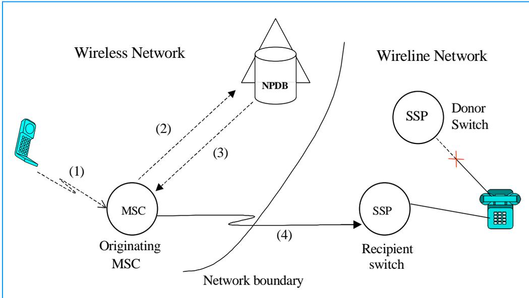
**Figure 2-14. Call Completion to Ported Wireline Number**
