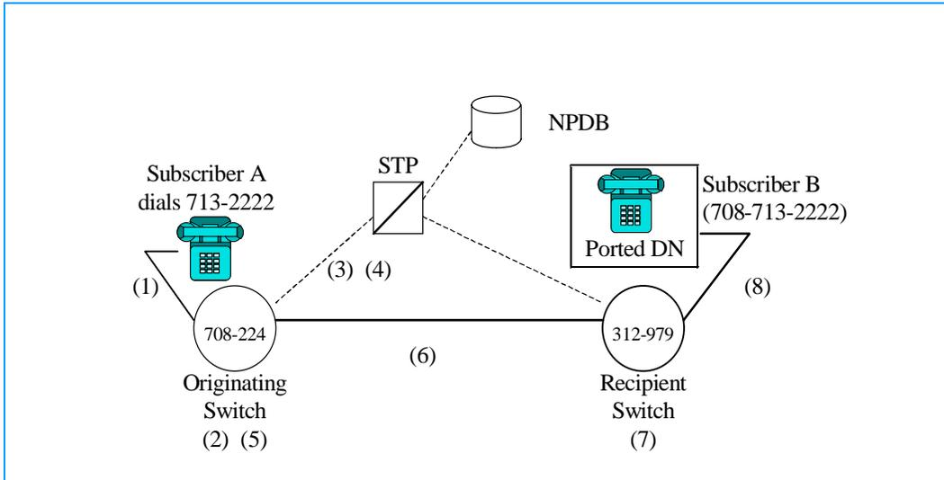
**Figure 2-9.** Originating Switch NP Processing with Direct Call Completion to the Recipient Switch
