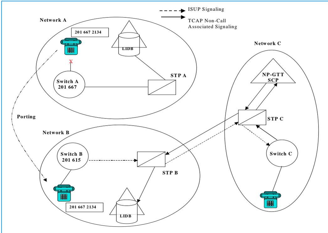
**Figure 2-8.** NP GTT Function in Support of Calling Name Delivery
