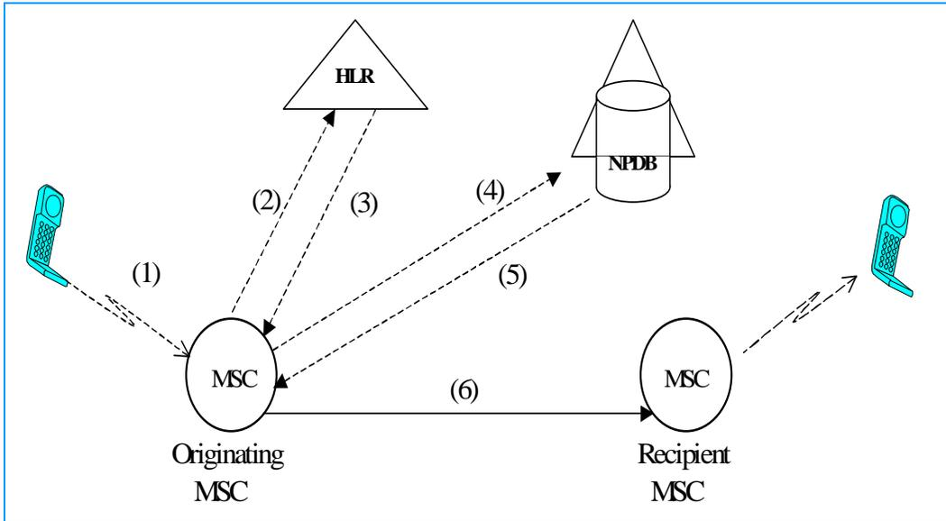
**Figure 2-16.** Call Completion after MIN/HLR Mismatch
