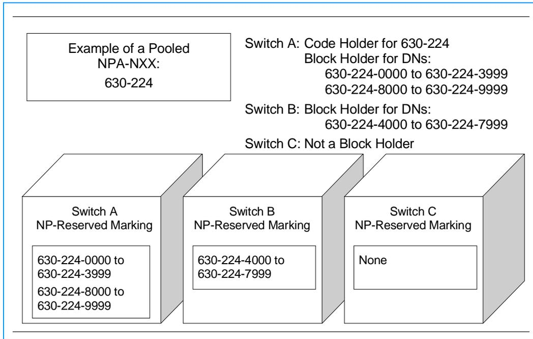
**Figure 3-5.** NP-Reserved Marking for Number Pooling
