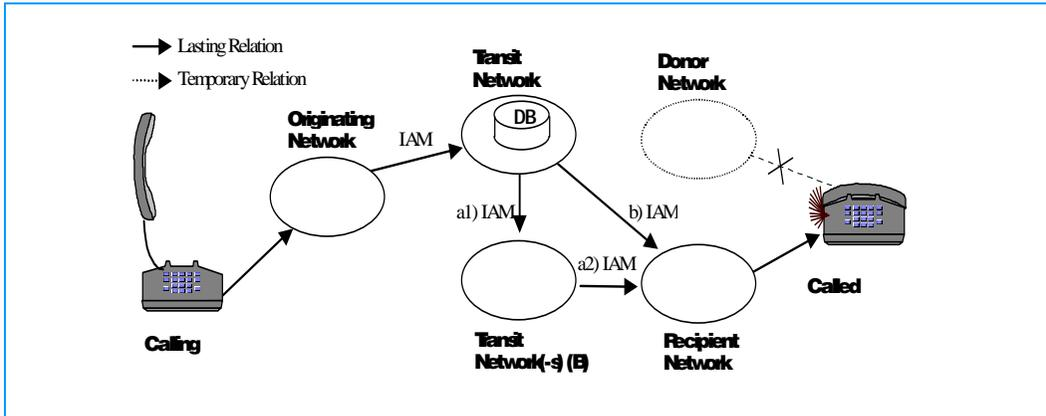
**Figure 2-18.** ITU Illustration of All Call Query “One Step” by a Transit Network
