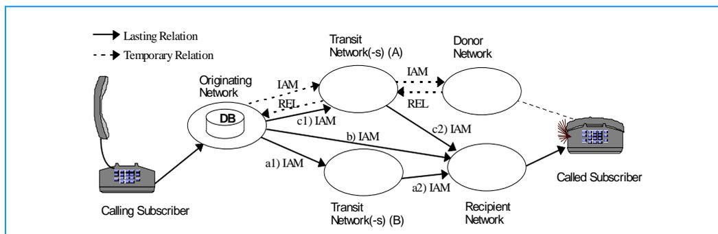
**Figure 2-20. ITU Illustration of Query on Release (Originating Network Query)**
