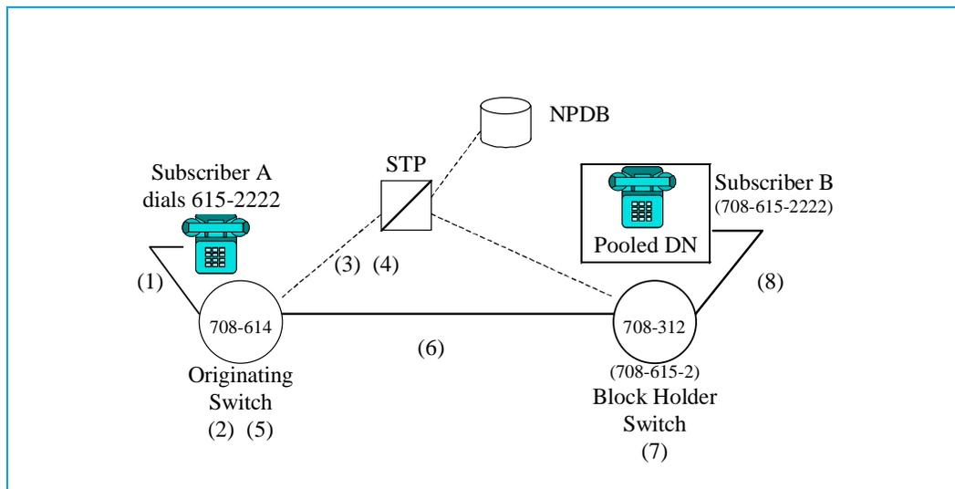
**Figure 3-6.** Direct Call Completion - Originating Switch to Block Holder Switch
