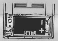
CAUTION: Install battery only in direction indicated or radio circuitry may be seriously damaged.
