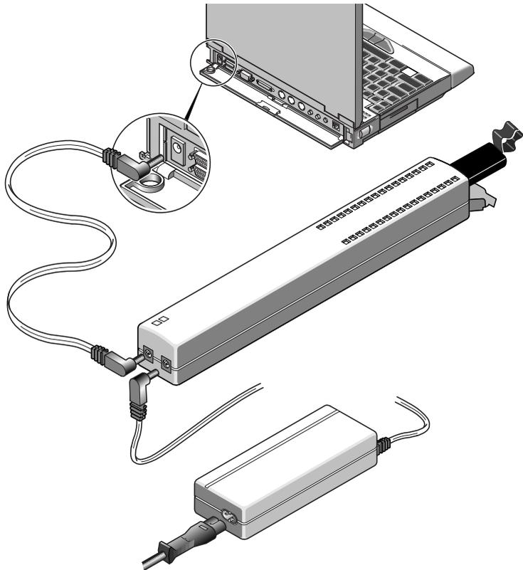
*Figure 4-3 Using the Battery Charger and Storage Unit*
