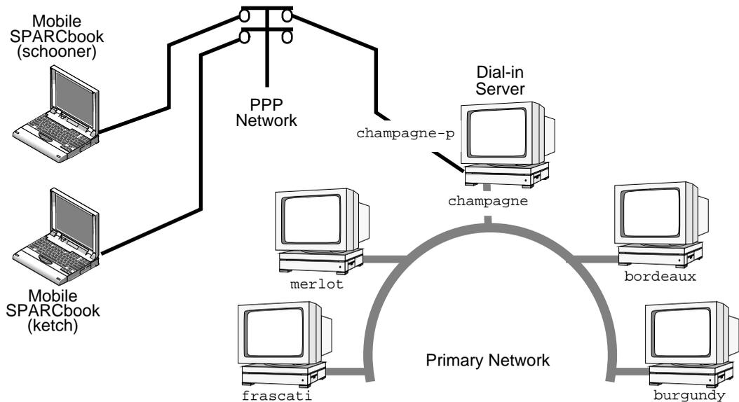
Figure 9-1 PPP Connection via a Dial-In Server
