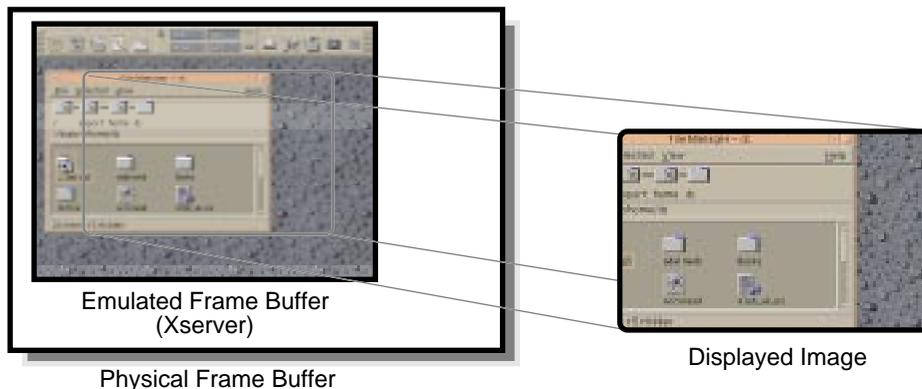
Figure 11-1 Xserver and Display Resolution
