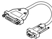
Figure 11-4 Sun Monitor Adapter Cable
