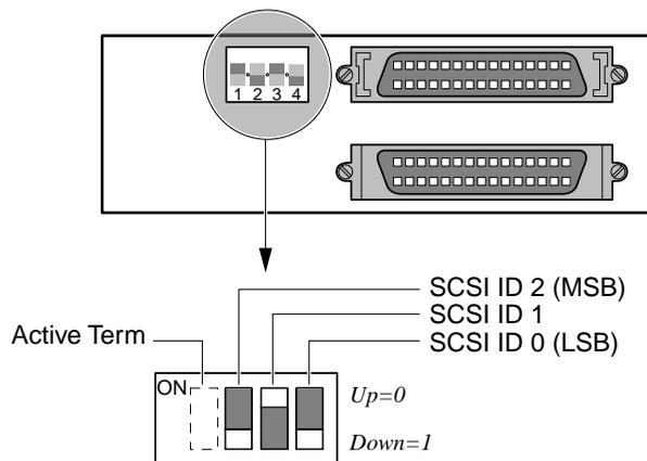
Figure 7-3 SCSI Floppy Disk Drive DIP Switches
