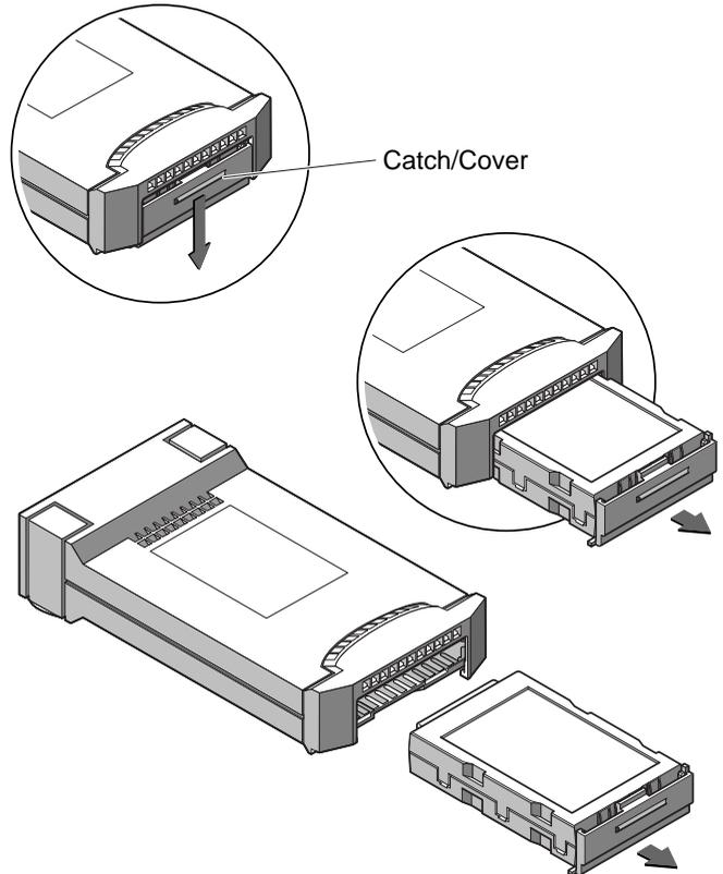
*Figure 6-4 Removing an RHDD From an Adapter*
