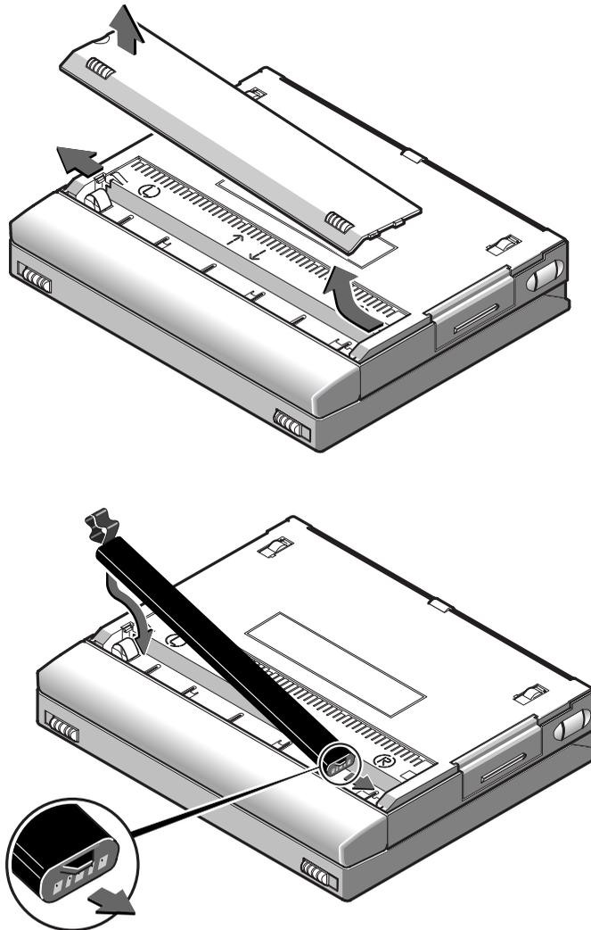
*Figure 1-1 Installing the Battery (SPARCbook 3000 Shown)*
