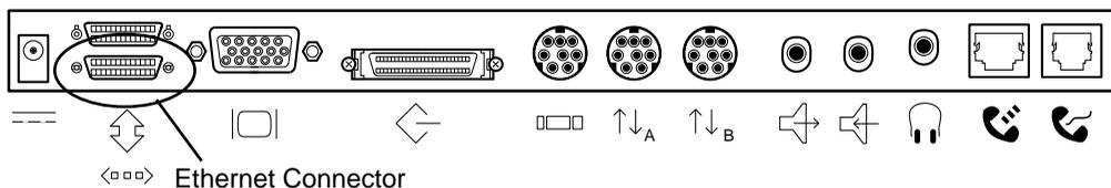
Figure 8-1 Ethernet Connector
