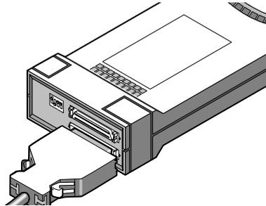
Figure 7-2 Connecting the SCSI Floppy Disk Drive
