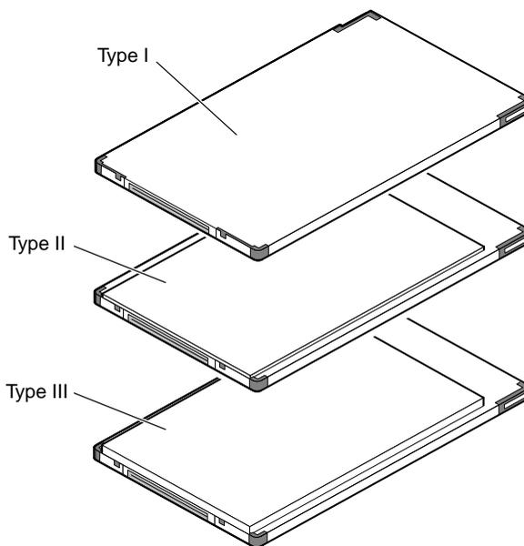
*Figure 10-1 PCMCIA Memory Cards and Peripheral Adapters*
