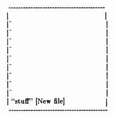
The cursor is in the top left hand corner with a row of tildes '~' down the left hand edge of the screen. The '~'s indicate that there are no lines in the file corresponding to these lines on the display. The bottom line displays the name of the file you are creating, and an indication that it is a new file.
