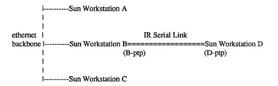
The /etc/hosts file or yellow pages (YP) host database needs to be set up as shown below. This allows the four workstations to share routing entries and work together. Notice that workstations A, B, and C are on the same net (192.9.200) and B-ptp, D-ptp, and D are on a second net (192.9.250).
