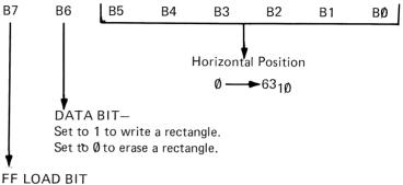
this bit should always =  $\emptyset$  for a horizontal position. When this bit equals  $\emptyset$  bit  $\emptyset$  — 6 are stored in the
