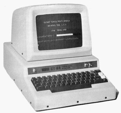
The CT-64 Terminal System kit is a low cost, ASCII stand alone computer terminal for use with either resident or remote computer systems. The display format of the CT-64 is 32 or 64 characters/line, 16 lines per page, 2 pages of storage and either page or scrolling operation with upper and lower case characters.
